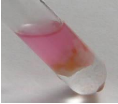
Example of a positive Fujiwara test
